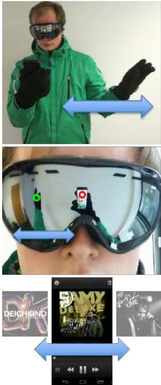
**Figure 4:** Top: Mid-air sliding gesture. GlassHands support large hand gestures, that enables continues scrolling or selection from a large list of options. Middle: Close-up with detected phone (red circle) and glove (green circle). Bottom: The album selection of a music player is operated with left and right sliding gestures.
