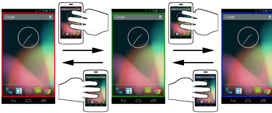
Fig. 4: The swipe switching mechanism allows to switch between zones with a three-finger swipe gesture. [best viewed in color]
