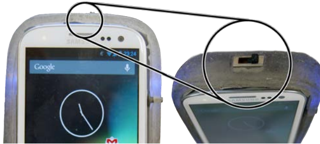
Fig. 5: The hardware switching mechanism utilizes the sliding switch mounted on the custom-built case to switch between zones. [best viewed in color]
