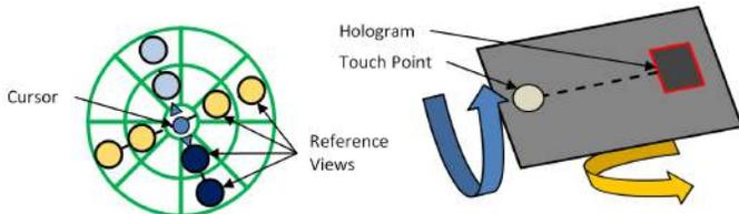
Fig. 10. Alternative layout of reference views (orientation) for hologram verification on movement paths. Reference views should be placed on a vertical path, making the device face towards the user in case the document is lying on a surface (dark-blue circles).
