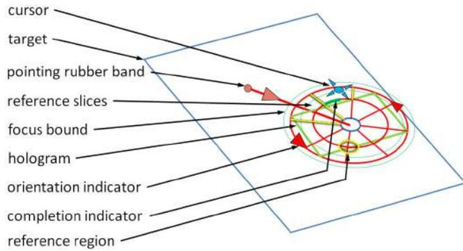
Fig. 7. Geometry of the proposed navigation approach for sampling a hologram. The user is guided to point at the element and a cursor is controlled by the 2D orientation on an augmented pie, divided into slices and tracks (constrained navigation). Alternatively, interesting subspaces can be indicated as circular regions instead of labeling relevant pie slices (hybrid approach).
