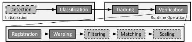
Fig. 2. Overview of our mobile hologram verification pipeline. For manual verification, images are registered and the extracted hologram patches are rectified. In case of semi-automatic verification, additional processing is required (dotted rectangles).
