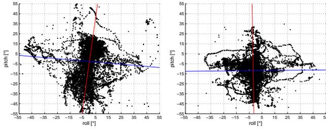
Fig. 9. Orientation changes during hologram inspection were considered with the document held in hand (left) and with the document kept on a table (right). This corresponds to tilting the document roughly in the vertical and also in the horizontal direction. In the first case, users did not move the document exactly in the vertical direction. This can also be seen by the visualized Eigenvectors (red and blue lines).
