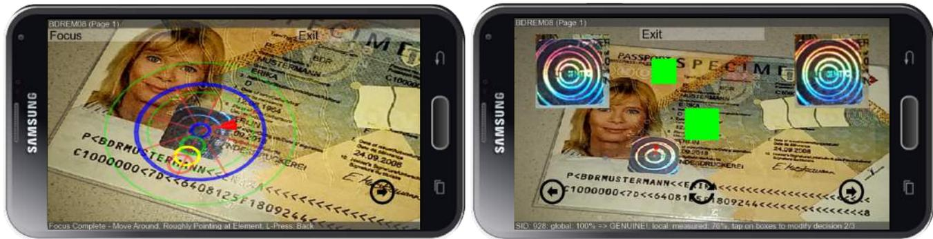
Fig. 1. Mobile prototype for hologram verification (specimen document): Hybrid user interface for capturing image data parametrized to indicate a constrained navigation space corresponding to typical user-behavior (left). Verification results are presented to the user in a summary (right).
