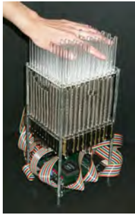
Figure 2: MATRIX [21], Multipurpose Array of Tactile Rods for Interactive eXpression, an array of tactile actuators
