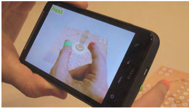
Figure 6: A green marker (thumb) and a red one (index finger) are used to track fingers and manipulate virtual objects on the board game. Source: [12]
