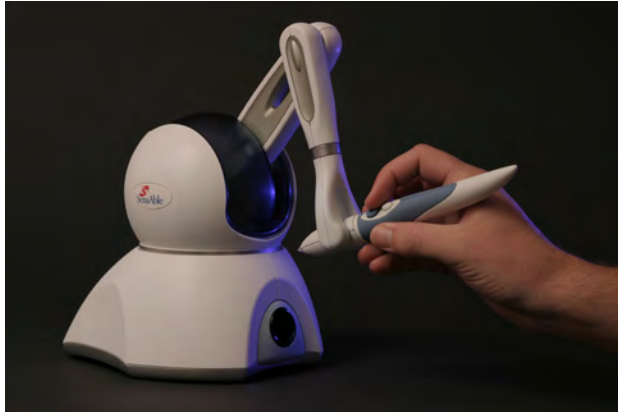
Figure 1: SensAble/Geomagic PHANTOM Omni Haptic Device 1 , providing force feedback to the user.
