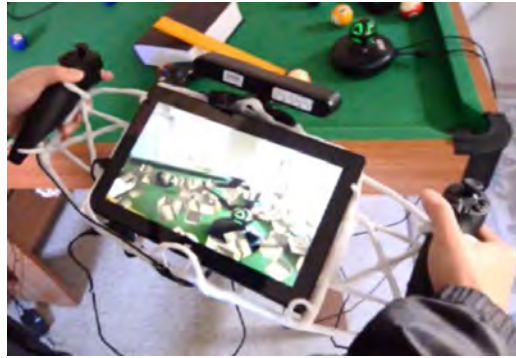
Figure 5: KITE Platform [22], hand-held AR device made with off-the-shelf hardware
