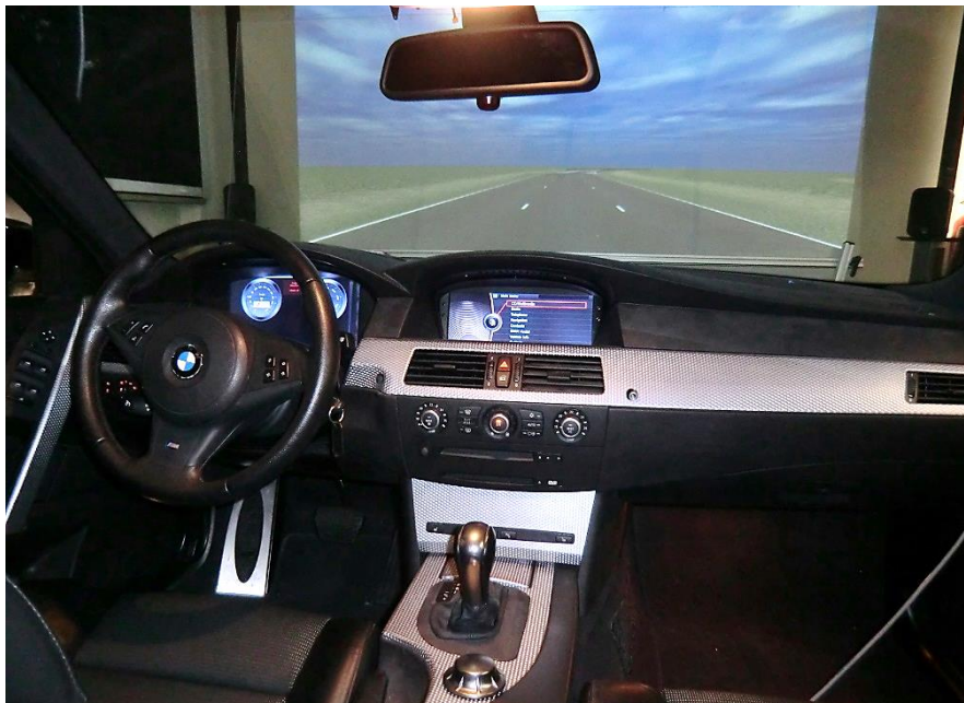
Fig. 3 The driving simulator used for the evaluation of the in-vehicle mode ( online mode ) of the framework. It is the real cockpit of a BMW 5-series. The framework controls parts of the dashboard and the display on top of the center stack, and can log most controls by monitoring the vehicle’s CAN bus.
