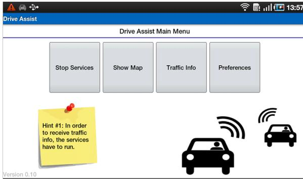
(a) *DriveAssist*'s main menu. The four big buttons in the top row are optimized for in-vehicle usage and allow controlling the central parts of the application. The yellow hint (bottom left) shows short pieces of usage information, when it is enabled in the preferences. The prototype runs on a 7 inch Samsung Galaxy Tab with Android 2.3.7.
