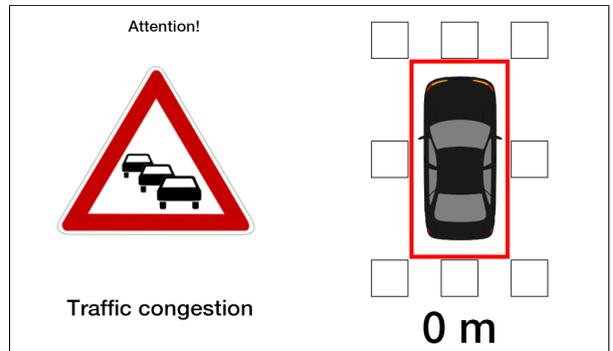
(d) When the traffic event is nearby (e.g. less than 15 meters away), the GPS accuracy may not allow indicating the precise position of the event. For that reason, the red border around the car shall symbolize the user that the event can be anywhere around the car.
