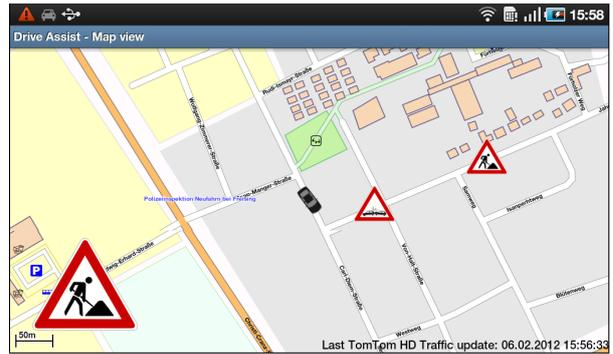
(b) *DriveAssist*'s map view. The black car in the center represents the driver's vehicle. The large traffic sign in the bottom left corner indicates the type of a newly received traffic event. The small traffic signs indicate the position as well as the type of the traffic event on the map.
