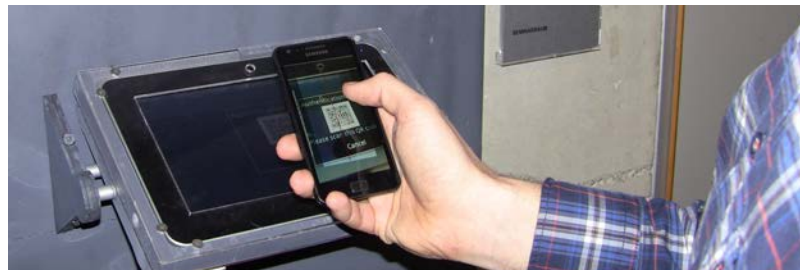
Fig. 6. Authentication at the door's entrance. The person is authenticated against the mounted interactive device with the smartphone. This allows the person to book an event, open the door and enter the room nearby (photo taken of a user during the login-process with out prototypical implementation).
