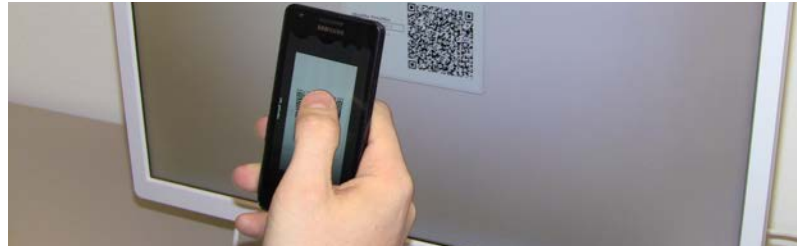
Fig. 7. The proposed login method for personal computer devices. The person in the picture using our prototype scans the time-limited QR code, which will provide username and permission to login to the service (e.g. to the login screen).
