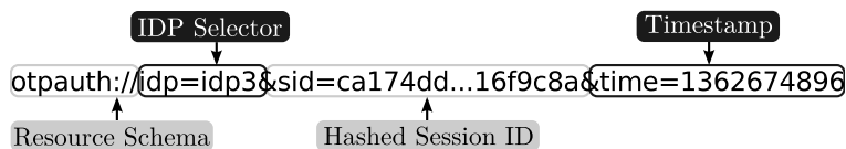
Fig. 2. Example structure of a Resource Identifier (URI) encoded in the QR code. The session ID is hashed using a secure hash function. For synchronization and validity estimation, the timestamp will be transported as well.
