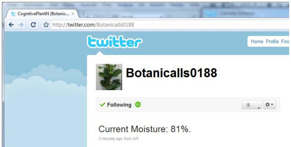
**Fig. 3.** The “Botanicalls” (<http://www.botanicalls.com>) device directly publishes e.g. moisture information to Twitter. This data is imported via a web service using the Twitter API into the ROS middleware and published to the plant care controller.
