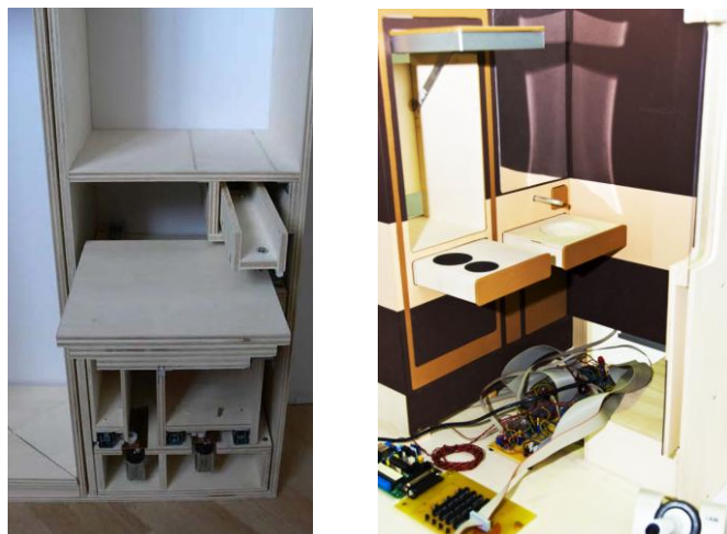
Figure 7. Left: 1:1 model of a Service Core “chassis”, customizable through modular and compatible sets of functionalities, smart appliances, sensors, actors, design fit outs. All functions can be automatically retracted into the core unit. Right: Sensor and actuator-equipped scale model of a service core with a model kitchen compartment (left) and hygiene area with functional water supply and sink (right).
