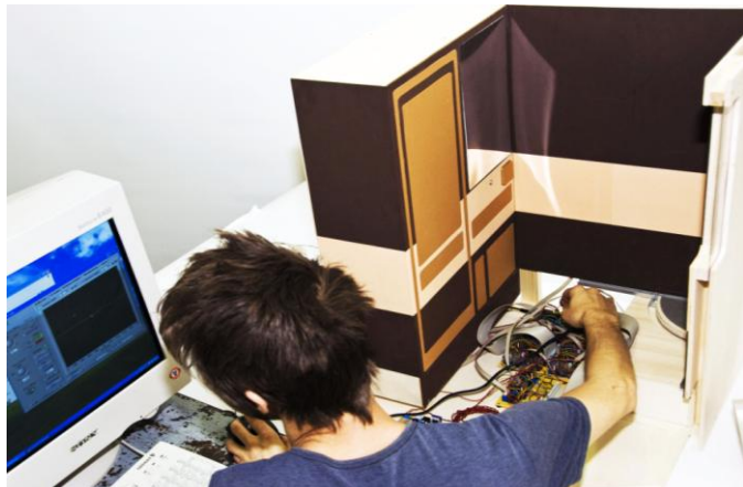
Figure 5. Fully functional experimental scale model and demonstrator, Scale 4:1. A room-in room type service core is shown. This example service core is an implementation of the functionality shown in Fig.2: bathroom, kitchen and sleeping room. The bed is hidden in the back wall, the bath room functionality is on the left wall behind and below the mirror, and the cooking functionality is in the left compartment of the left wall.
