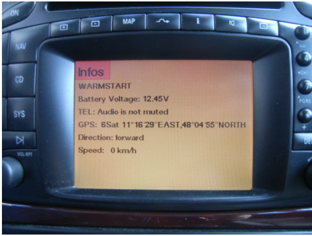
Figure 3: Debug Information System: The debug information system of the Mercedes G400 delivers battery and audio status, the coordinates as measured by the in-vehicle navigation unit, the driving direction as set by the automatic gear and the current speed as measured by the odometry.
