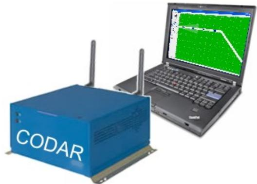
Fig. 4. Simulation Setup: CODAR OBU +  $m^3$  Simulation Laptop
