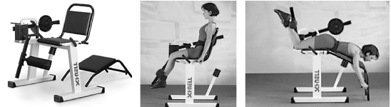
Fig. 1. The Synchronous Training Machine: the gear box on the axis does not allow for sensor inclusion. No sensor system from the sports equipment manufacturer can be obtained, which is true for many other systems as well. This is just an example of many expensive sports devices that can be augmented by our proposed sensing system.
