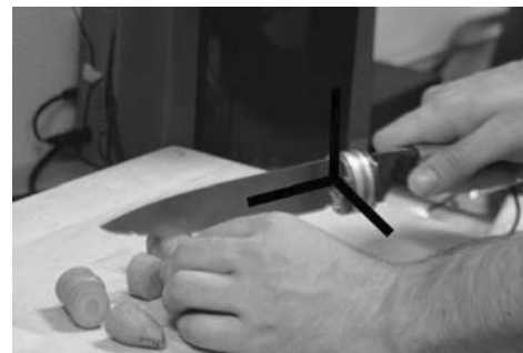
Fig. 9. Instrumented knife cutting carrots. A three axis force/torque sensor has been soldered between handle and blade. The weight of the sensor is minimal and nearly unnoticeable. The three axes are drawn as black lines in the image above. The sensor does not hinder normal “operation”.
